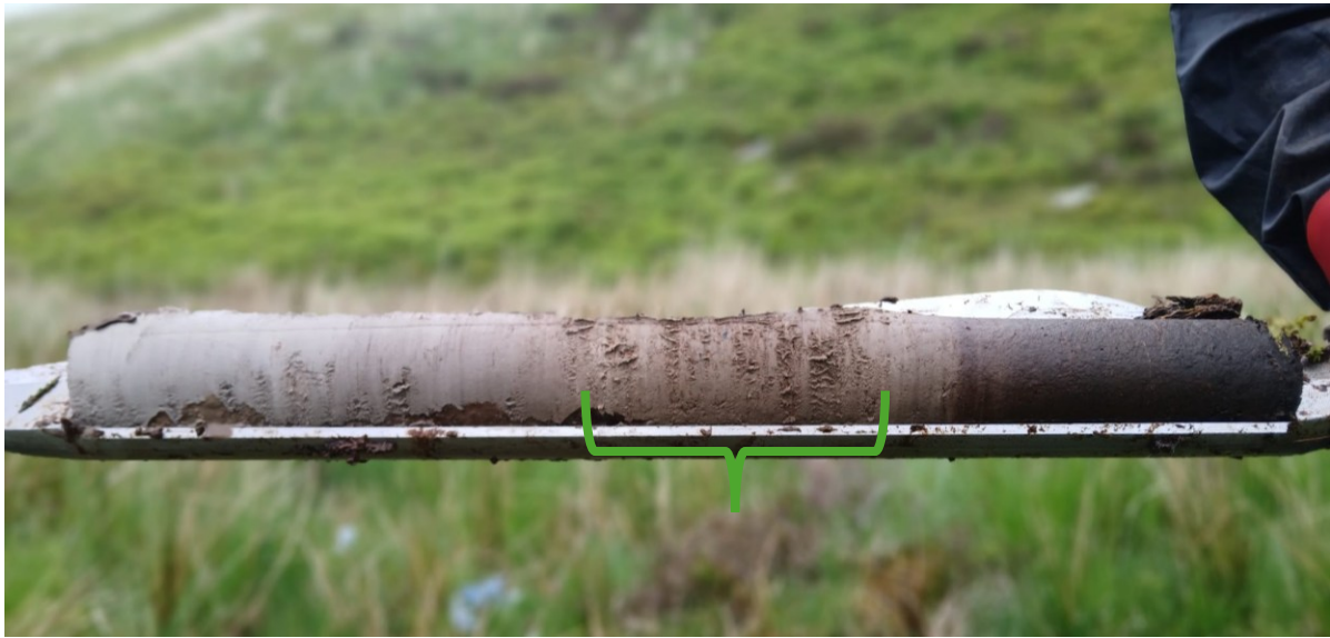
Figure 5: Field photo showing potential tripartite sequence transitioning into blue grey clay, expected to align with glacial conditions.
