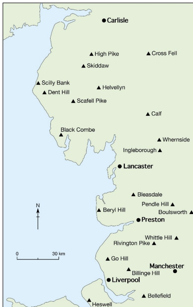
Figure 1. Outline map of northwest England showing locations of sites from which triangulation observations were made in 1807-08 and the 1840s and used in the Principal Triangulation of Great Britain.
